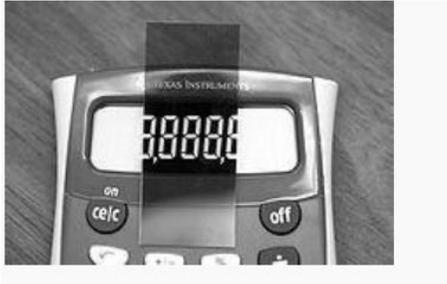
LCD with top polarizer removed from device and placed on top, such that the top and bottom polarizers are parallel.
