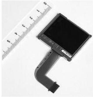
A Casio 1.8 in colour TFT liquid crystal display which equips the SonyCyber-shot DSC-P93A
